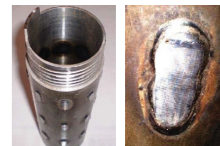
Obsolete locking coupling with tang & hard facing wear pad detail
