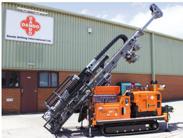
Above: the Multitec 4000 was designed for Dando customers requiring a small, affordable rig that could take samples to 200m
